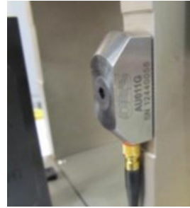
Typical Piezo Strain Sensor Mounting locations Steel Frame and Cast Iron Frame Presses
