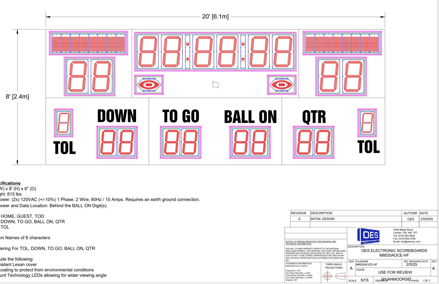
Overall size: 20' (W) x 8' (H) x 6" (D) Approximate Weight: 815 lbs Incoming Mains Power: (2x) 120VAC (+/-10%) 1 Phase, 2 Wire, 60Hz / 15 Amps. Requires an earth ground connection. Incoming Mains Power and Data Location: Behind the BALL ON Digit(s).
